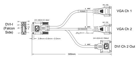
A31-00735-1012 (VLG-3/1) cable assembly for /T version
