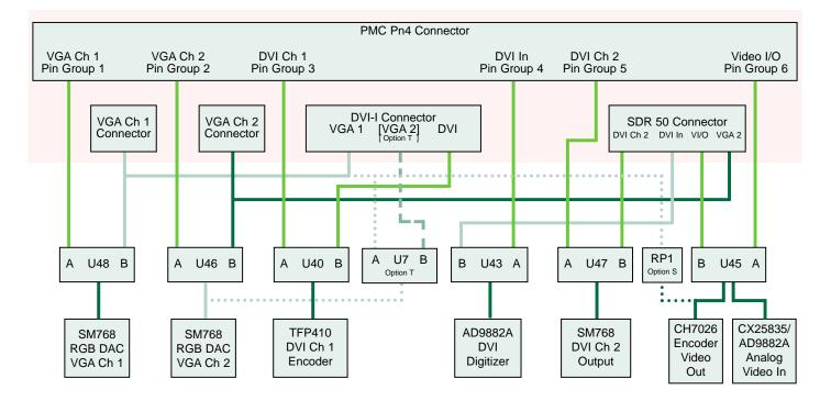
Options S and T are shown for completeness and are used only in customer special builds
